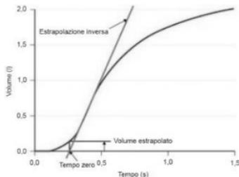
$$\text{Nullzeit} = t_{\text{PEF}} - (V_{\text{PEF}}/\text{PEF})$$
