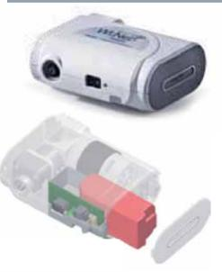
Due to its innovative technology Wi.Neb has reached a so far unequalled mix of power, compact size and lightness. The **Lithium-Power battery** does not require special maintenance. Located inside the unit, it is easily accessible by removing the side cover. The **PWM (Pulse Width Modulation)** technology ensures a constant delivery during battery operation. The battery pack can be fully charged in about 2 hours through mains supply or through the 12V cigarette lighter power cable.
