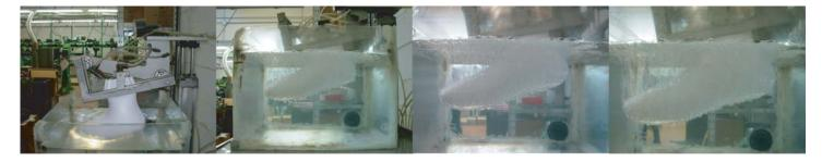
The air bubbles come out continuously from the sock showing the high wicking of **MICROAIR**<sup>®</sup> *IN-Between* barrier fabric; furthermore, the inside of the sock is perfectly dry prooving that both the barrier fabric and the seams are totally waterproof.
